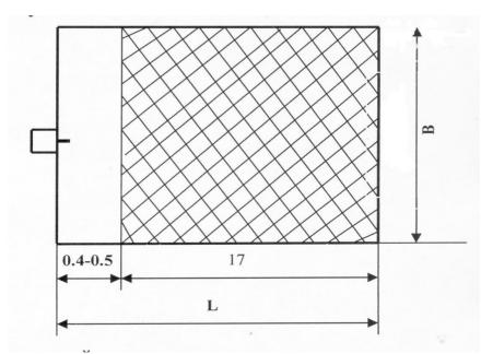
The distance from the nozzle to the perimeter of the protected area shall be 0.4-0.5 m. Nozzle location height  $\leq$  3.9 m.
